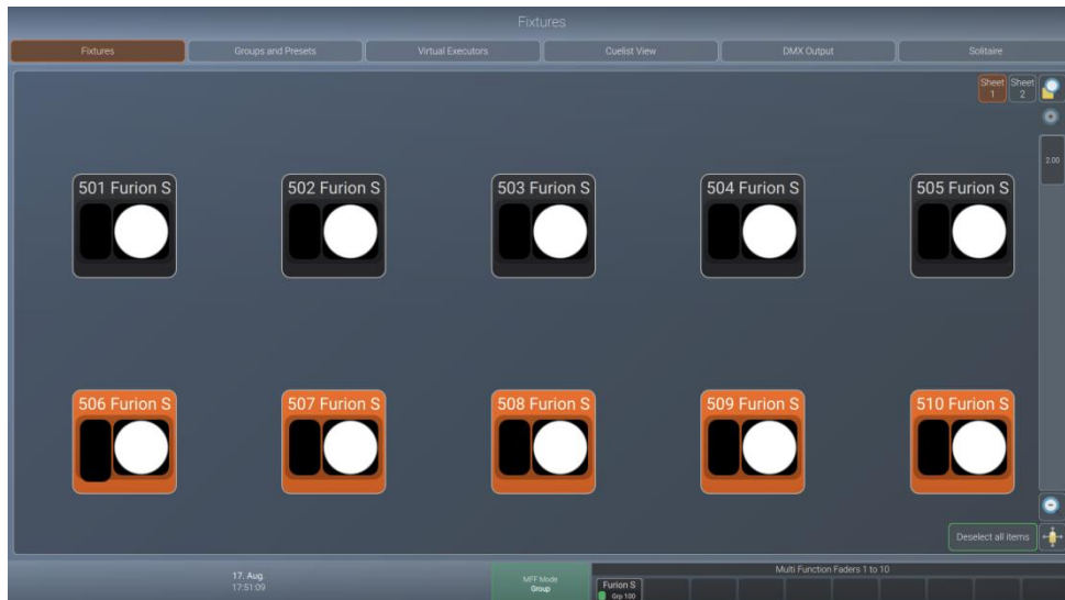
Fig. 21: External Monitor Fixtures View – LAMPY DNGL attached
