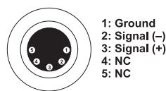
DMX-output XLR mounting-socket:
