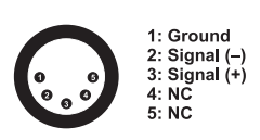
DMX-input XLR mounting-plug:
