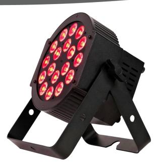
The ADJ 18P Hex is an all metal, powerful 216W LED Par fixture with 18x 12-Watt, 6-IN-1 HEX LEDs. With a 25-degree beam angle, users may produce wide washes with smooth color mixing from 63 built-in color macros utilizing red, green, blue, amber, white and UV LEDs. Not only is this LED Par great for lighting stages, but with its patent pending, intelligently designed, power and DMX connectors, it's great for uplighting large venue.
