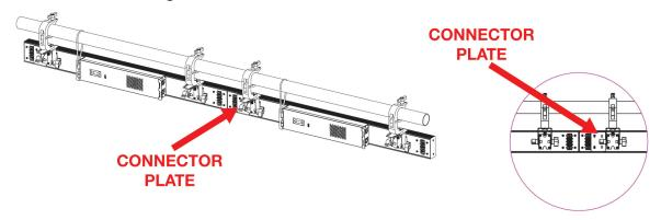
2. Remove the two (2) screws holding the connector plate in place, as well as two (2) screws on the end of each adjacent unit, for a total of six (6) screws. Remove the connector plate.
