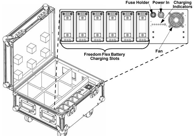
The Freedom Flex Case is an auto-ranging power supply and it can work with an input voltage range of 100 to 240 VAC, 50/60 Hz.
