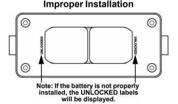
The tabs on the Freedom Flex Battery will be fully extended when it is properly installed. Ensure the Freedom Flex Battery is properly installed to preserve the product's IP rating.
