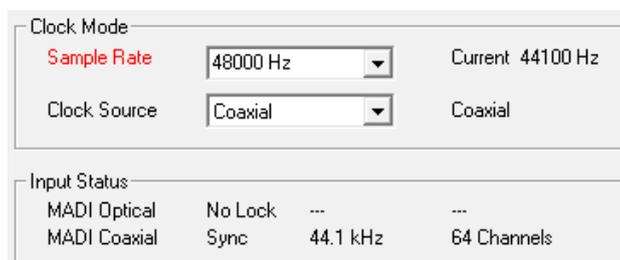
The screenshot shows the 'Clock Mode' section with a 'Sample Rate' dropdown set to '48000 Hz' (highlighted in red) and a 'Current' value of '44100 Hz'. The 'Clock Source' dropdown is set to 'Coaxial' with a 'Current' value of 'Coaxial'. Below this is the 'Input Status' table:
