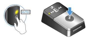
▶ To unmute the audio signal: Briefly press the button on the transmitter or the pedal switch on the receiver.
