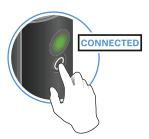
▶ To mute the audio signal: Briefly press the button on the transmitter or receiver.
