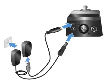
Connect the receiver to the power supply system. You can use the included power supply unit or power the receiver via the USB port. Battery operation is not possible.
