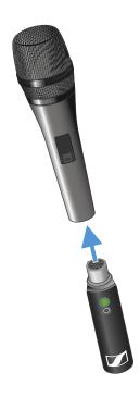
▶ Plug the transmitter into the XLR socket on your microphone.
