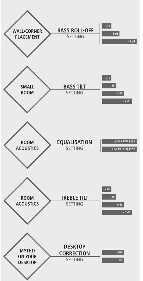
The low frequency attenuation is necessary when loudspeakers are placed near the room walls or corners. The amount will depend on the specific situation (in general -3 dB for wall placement and -6dB in case of corner placement).
